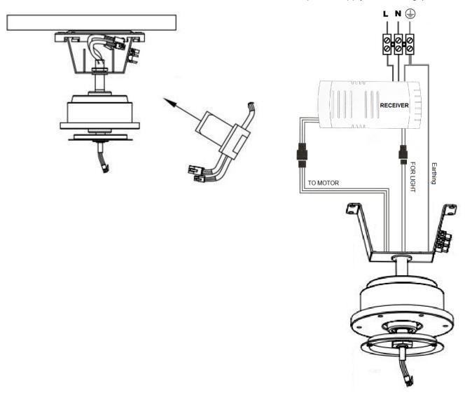
3. Set up the remote receiver on the motor U-frame. Wiring according to remote control wiring diagram.
