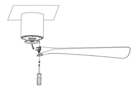
5. Fasten the blade to the fan-motor assembly by the blade bracket screws.
