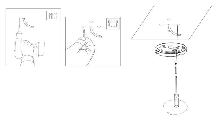
1. install the Slide-in mounting bracket tray to the ceiling. (please ensure the fixing is able to support minimum moving weight of the fan which is 15.8kg=35Lb)
