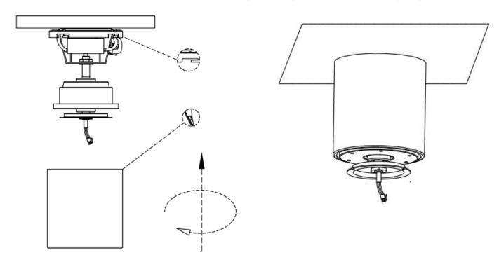
4. Carefully fit the Fan motor enclosure into the motor assembly and align the locking slots of the Fan motor enclosure with the four locking slots on the mounting support tray. Push upward into the locking slot and turn clockwise to lock into place.
