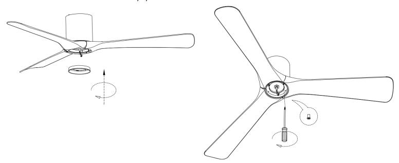
6.Remove the three screws from the fan - motor assembly. Align the three holes in the light kit pan Make sure the notch in the light kit pan and re-install the three screws that were removed in the first step to secure the light kit pan.
