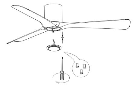
7. Connect the 2-pin plug exiting the bottom of the fan motor to the 2-pin plug from the LED light kit pan. Secure the LED light kit in the light kit pan .
