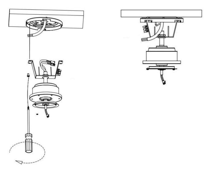
2. Carefully lift the fan-motor assembly up to the Slide-in mounting bracket tray. Install the fan-motor assembly using the 4 mounting screws on the slide-in mounting bracket tray.
